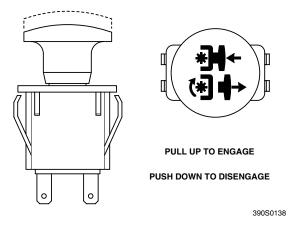
Figure 4-3. Cutter Engage Switch
